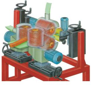
**Model QT4** is as QT2 but with two horizontal sanding drums also equipped with Quick Flex. The lower sanding drums are fixed in the table and the upper ones are adjustable up and down.
