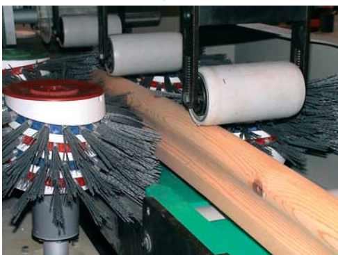
Wood cleaning with QN Tynex
