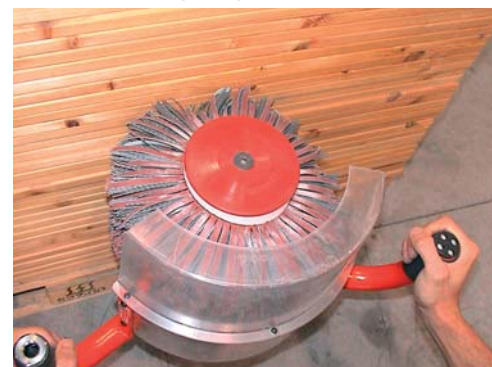
Sanding of edges with QN + QD
