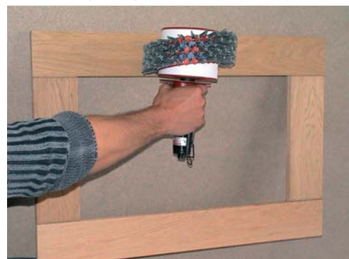
Rustic grooving of soft wood with QN Tynex
