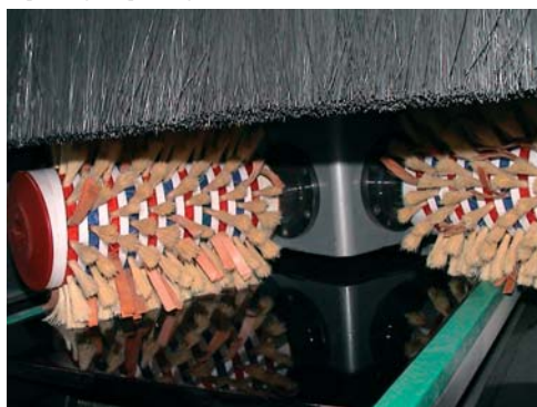
Spreading and polishing wax on the surface with QN Sisal and Leather
